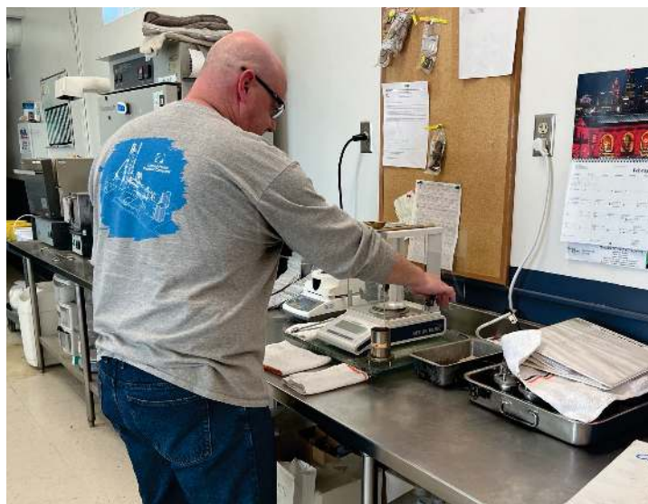
A Quality Control Technician weighing 325 sieve material with balance at the Kansas City Performance Center lab in Sugar Creek, MO.
